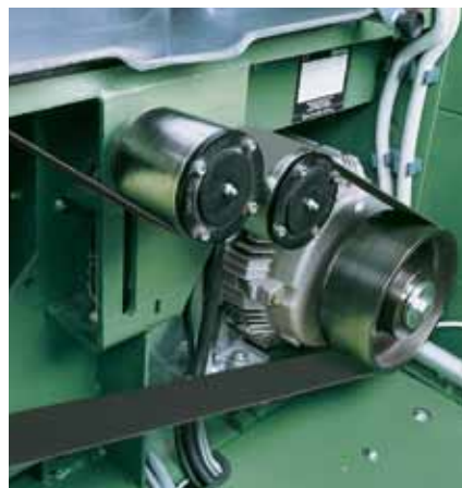
Drive (textile industry/yarn manufacture), belt type GG 20E-20 NSTR/FSTR grey/black
