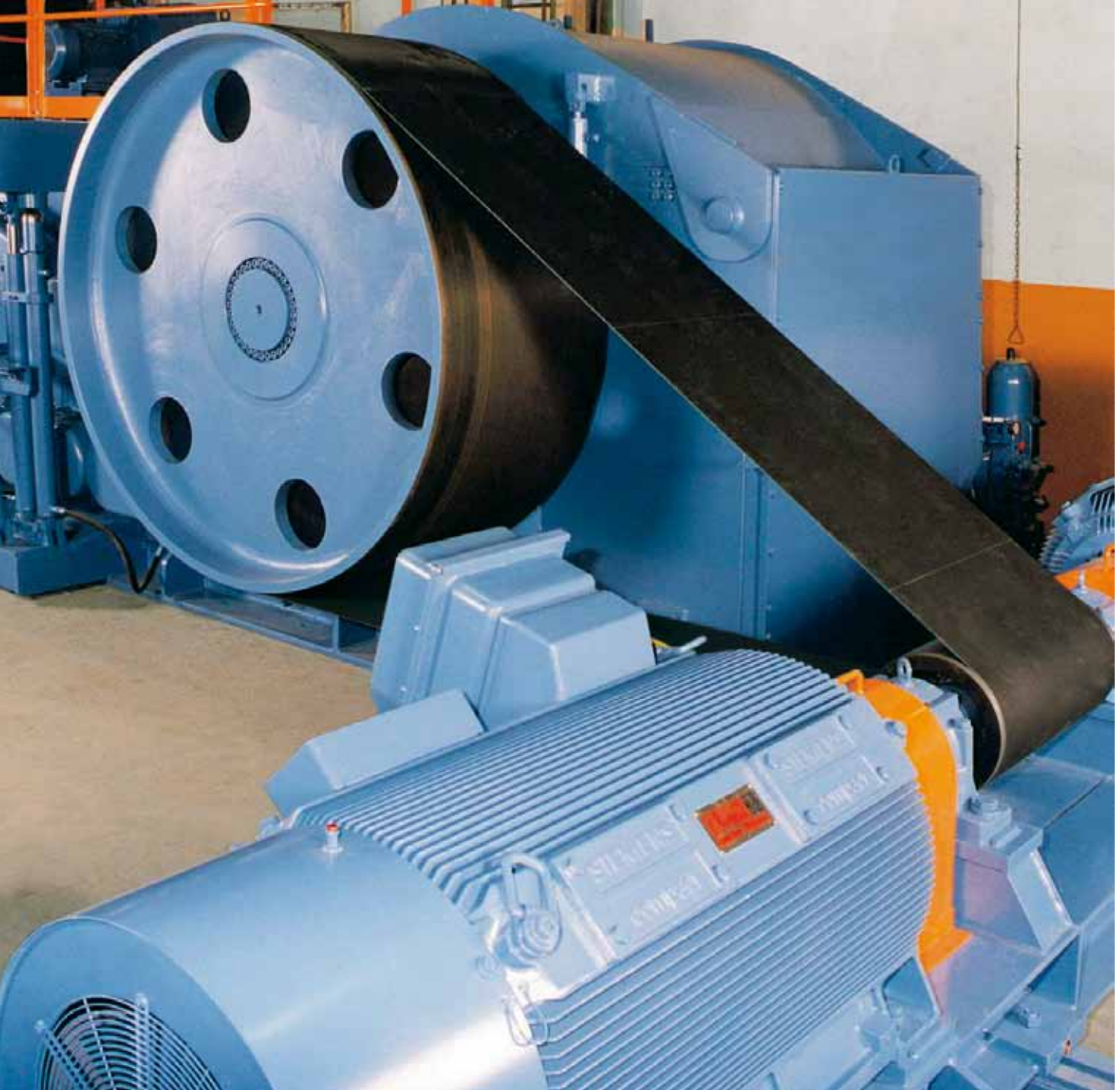
Chipper (wood manufacture), belt type GT 80 P black, width = 1000 mm, P = 1850 kW, v = 65 m/s
