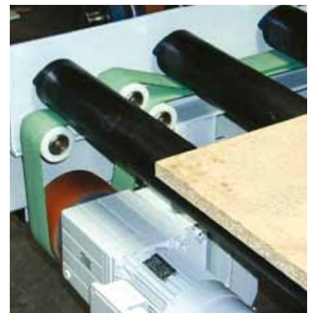
Live roller conveyor (logistics), belt type GG 20E-20 green
