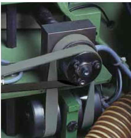
Drive (textile industry/yarn manufacture), belt type GG 20E-20 NSTR/FSTR grey/black
